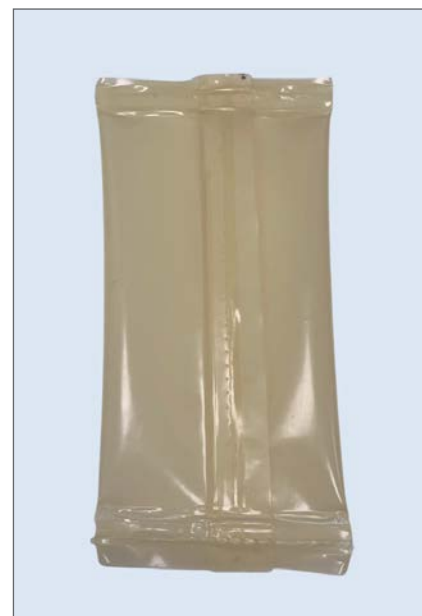
Figure 2 Illustration of a flow pack obtained from casein fraction recovered from expired milk
